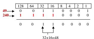
Result of above AND operation is zero 48 hence the first IP address is 192.168.10.48
