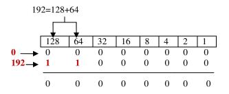
Result of above AND operation is zero (0) hence the first IP address is 192.168.10.0
